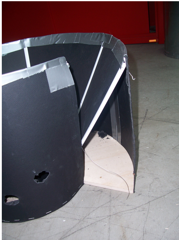
Figure A.9 Side view of inverted cone installation for spiral chamber floor Design modification and fabrication by J. Pierce Scarlett, photo courtesy J. Pierce Scarlett
